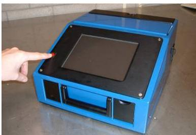
3. The 8 inch touch screen should be handled with care. Do not operate the screen with sharp objects. Do not use any chemicals or fluids to clean the screen, but use a dust free cloth. Simply press the red power button to switch the Proliner on and off.
